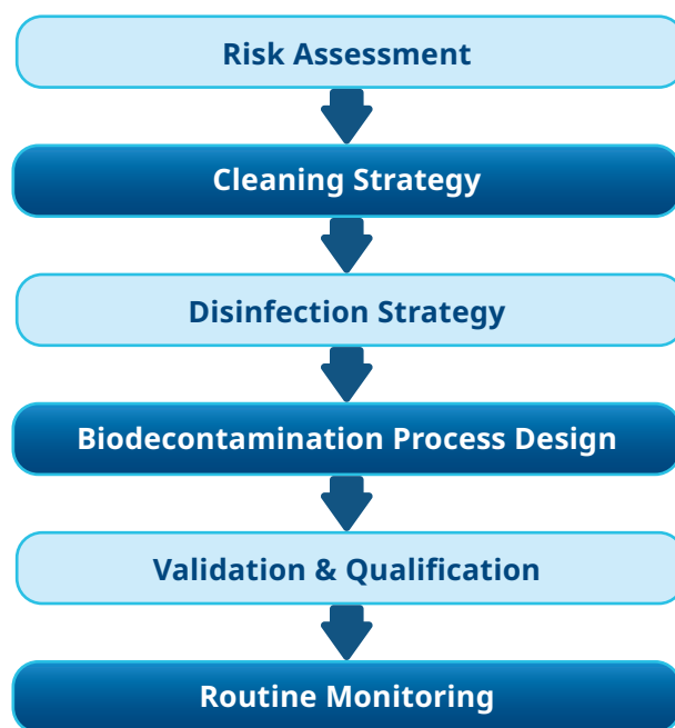
Figure 4. Lifecycle framework for bio-decontamination control within a Contamination Control Strategy.
